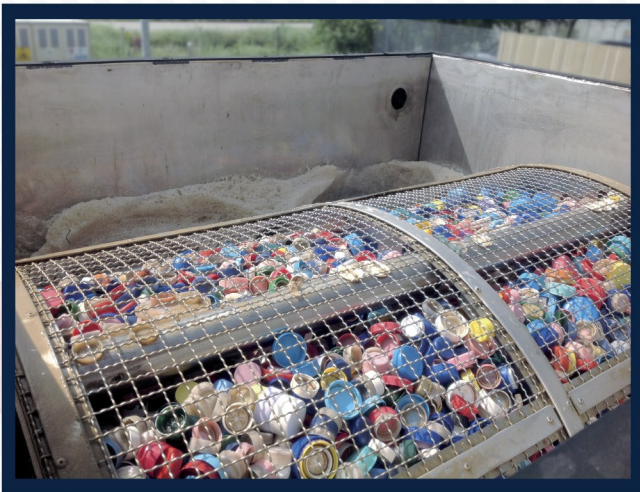
Fig. 1 - The reaction cell is partially (40%) plunged in the sewage and partially exposed (60%) to the air by slow and constant rotation of the cell. Heterotrophic and autotrophic ( Nitrosomonas spp , Nitrobacter spp ) bacteria grow as biofilm on the carriers in a week time promoting both carbon removal and ammonia oxidation.
